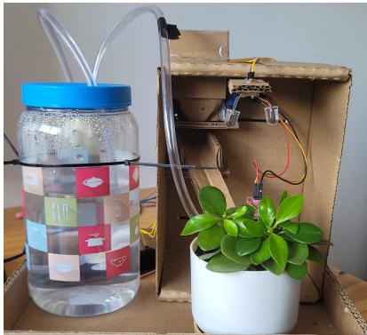
Fig. 6. Prototype hardware being used in a plant
