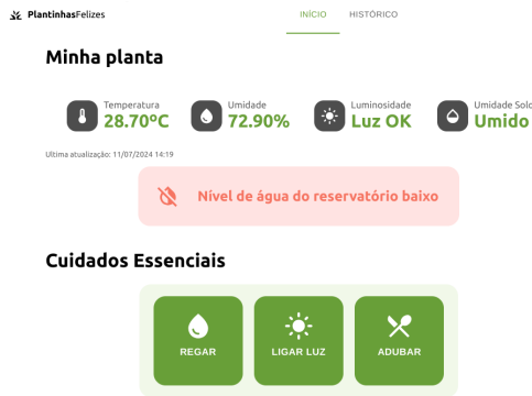
Fig. 7. First screen of the web application with buttons for actuators and visualization of the last reading taken by the sensors
